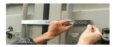
The two barriers should be blocked the closest possible in order to avoid any opening of the container.
