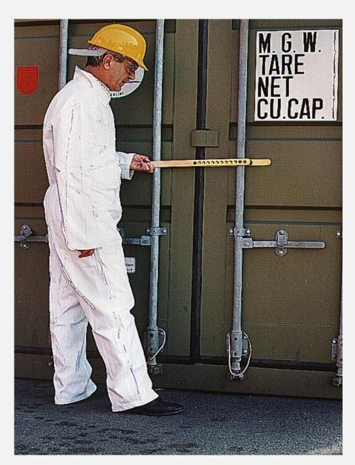
This security seal acts by clamping the two central barriers of the container and clearly blocking the doors opening.
