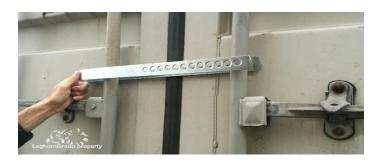
Insert the Forkseal between the two central barriers of the container, ensuring that the bend part of the barrier seal matches perfectly with the left barrier of the container.
