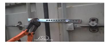
Once we reach our destination, a bolt cutter is necessary to remove the FORKSEAL and free the doors of the container.
