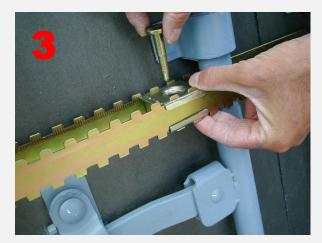
4.) ... Insert the bolt lock and set off the locking mechanism. FROM THIS POINT FORWARD, THERE IS NO POSSIBILITY OF TAMPERING.
