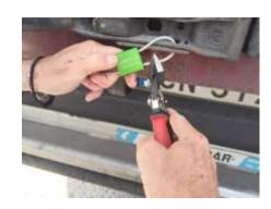
To remove the seal, special cutters are required.
